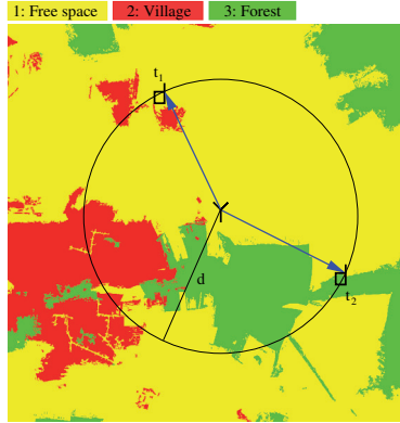
Figure 3.2: In the Erceg model, receivers t_1 and t_2 experience equal path losses due to the same distance d and the same predominant terrain type.
