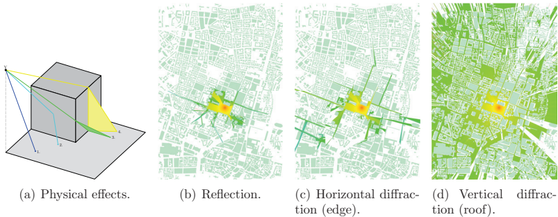
Figure 3.3: Visualization of the modeled physical effects on launched rays.
