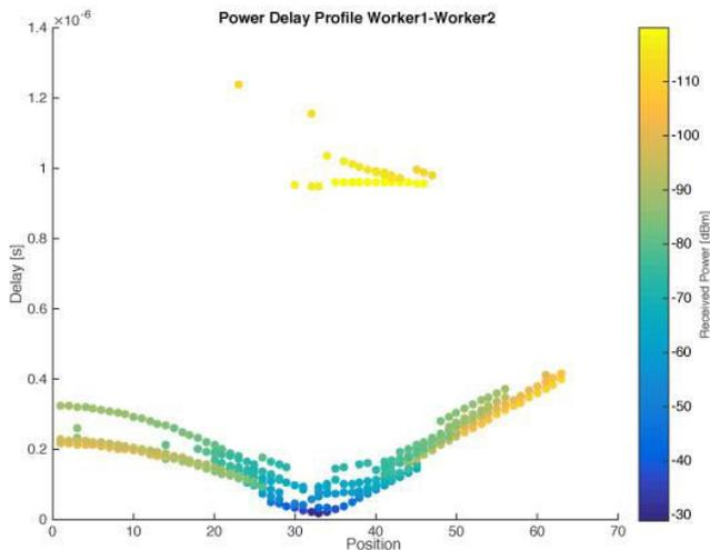
Figure 4. Worker 1-Worker 2 power-delay profile. (Source: Own)
