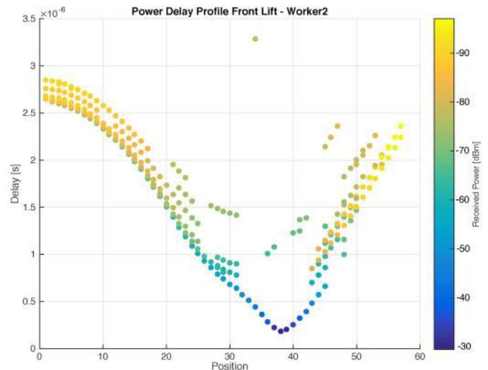
Figure 2. Front forklift-Worker 2 power-delay profile. (Source: Own)
