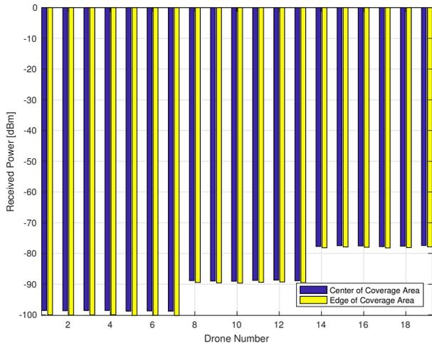
Fig. 5. SNR at the center and at the edge of each coverage region.
