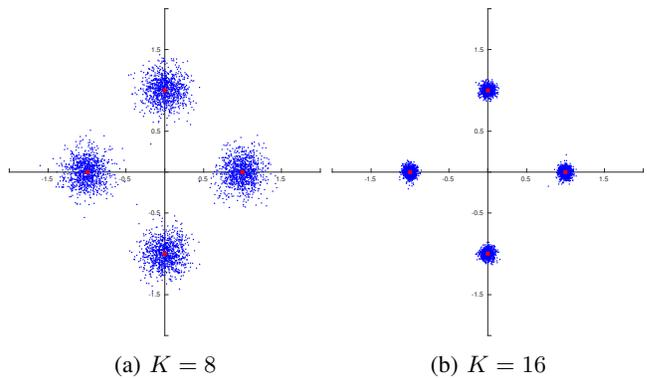
Fig. 3: Estimation of target signals with proposed estimator ( $L = 4$ ,  $P_k = 2$ ,  $P_{\text{tot}} = 10$ ,  $\sigma_s = \sigma_c = 0.1$ ,  $\text{SNR} \approx 20$  dB). Estimation is done for 1000 estimation instances (different realizations) whose estimation values are shown with blue dots, while the red dots correspond to the constellation points of target signals.
