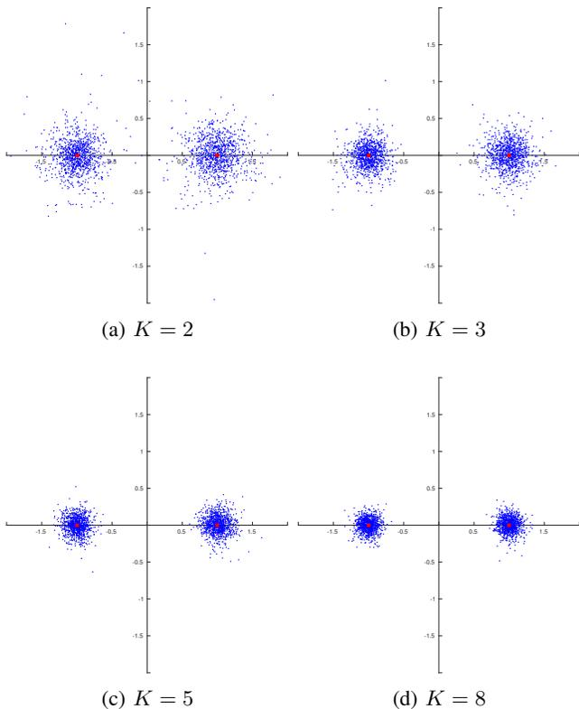
Fig. 2: Estimation of target signals with proposed estimator ( $L = 2$ ,  $P_k = 2$ ,  $P_{\text{tot}} = 10$ ,  $\sigma_s = \sigma_c = 0.2$ ,  $\text{SNR} \approx 14$  dB). Estimation is done for 1000 estimation instances (different realizations) whose estimation values are shown with blue dots, while the red dots correspond to the constellation points of target signals.
