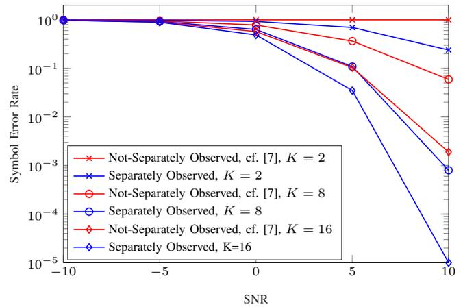
Fig. 5: SER against different values of SNR for several numbers of sensors  $K$ . It is assumed that  $L = 4$ ,  $P_k = 2$ ,  $P_{\text{tot}} = 10$ . The blue lines correspond to the system of the current paper, while red lines represent SER of a system whose sensor nodes cannot separately observe the targets, [7]. Power allocation is performed in both cases.
