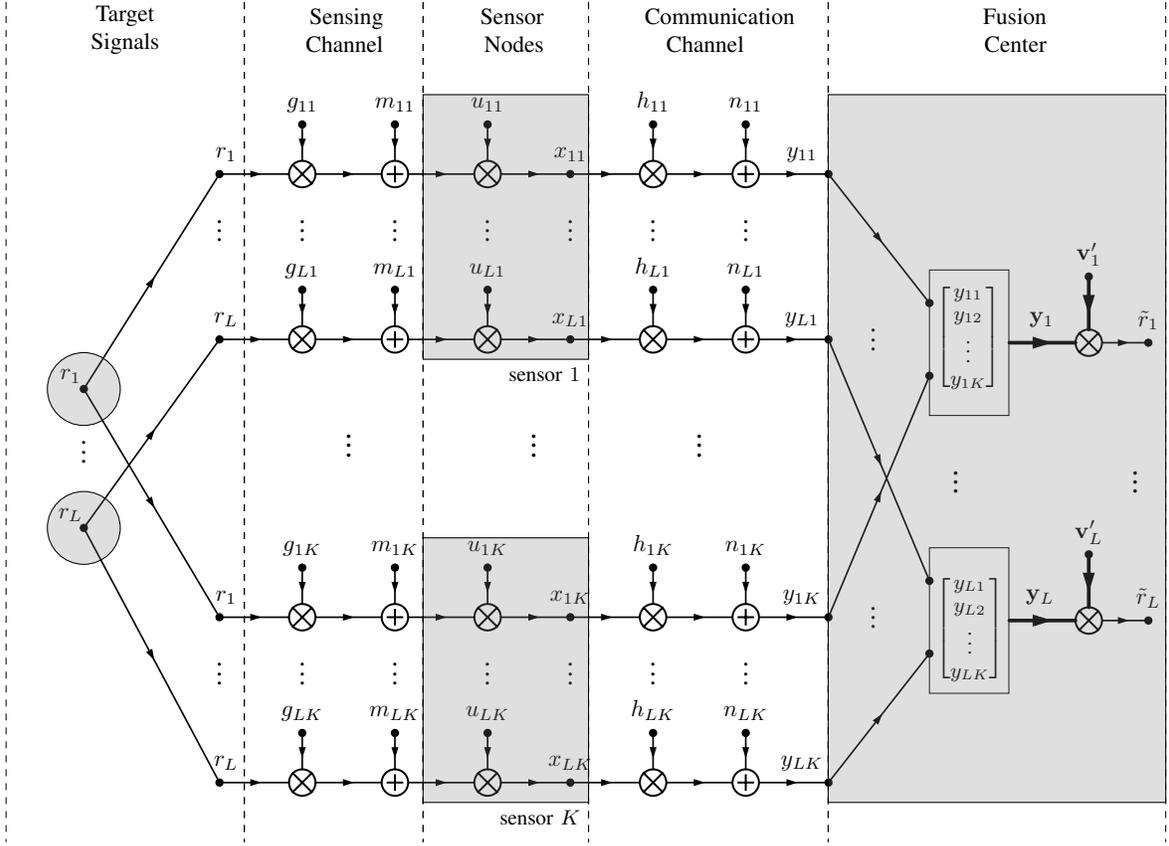
Fig. 1: Block diagram of the multi-target wireless sensor network. Targets are observed separately at each sensor node and fused separately at the fusion center.
