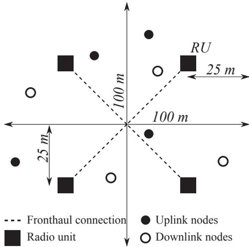
Fig. 2. The simulated setup. RUs are located at the center of each small square ( $50 \times 50$ ), where the position of the UL and DL users are chosen randomly.
