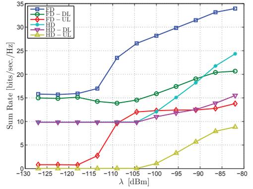
Fig. 4. Sum rate [bits/sec./Hz] vs. tolerable interference threshold at the PUs  $\lambda$  [dBm].
