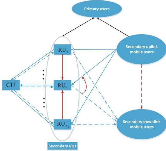
Fig. 1. Full-duplex cognitive cloud radio access network. The solid and dashed lines refer to uplink and downlink transmission, respectively.
