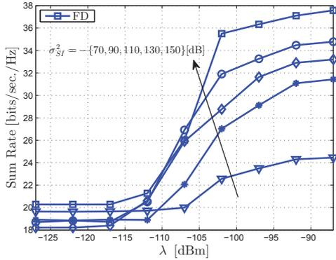
Fig. 5. The impact of the self-interference channel  $\sigma_{SI}^2$  is depicted for different values of  $\lambda$  [dBm].
