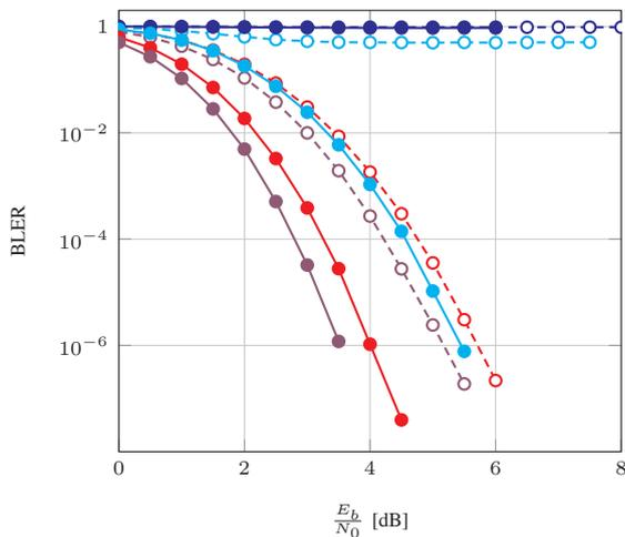
Fig. 3. Catastrophic performance degradation under SC decoding due to incapable positions included in  $\mathcal{A}$ . The index set  $\mathcal{A}$  is selected based on a DE taking into account the puncturing pattern  $\mathcal{P}_3$ . Please see Figure 2 for legend.
