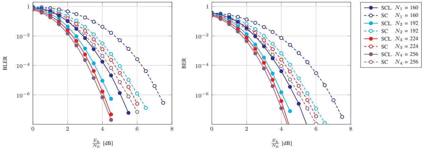
Fig. 2. Performance of the codes  $\mathcal{C}_t \in \mathcal{C}$  under SC and SCL decoding. All codes are of dimension  $K = 96$ , and are obtained via appropriately puncturing a mother PC of length  $N = 256$  using QUP and the parameters given in Table I. The index set  $\mathcal{A}$  is selected based on a DE taking into account the pattern  $\mathcal{P}_1$  of cardinality  $|\mathcal{P}_1| = 96$ .
