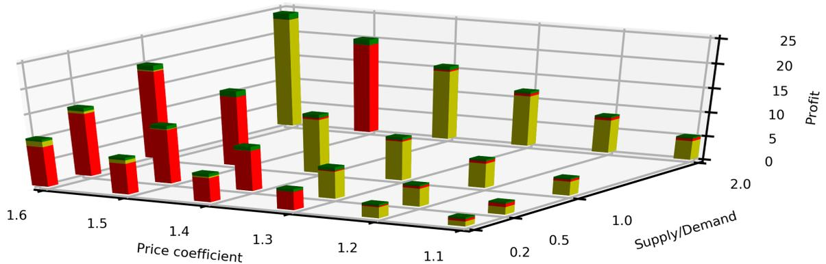
Fig. 3. Table and graph with average expected profits of the optimal solution (green), expected best-pair heuristic (red) and the optimal solution not considering the choices (yellow) for different travel prices and supply/demand ratios. The simulation was run 100 times for each case.
