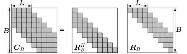
Fig. 1. Cholesky decomposition. The band structure of  $\mathbf{C}_B$  is retained in the Cholesky factors. The Toeplitz structure is not.
