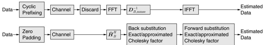
Fig. 2. Block transmission systems using zero padding and LS/MMSE estimation on the basis of either circulant or rectangular submatrices. We also apply the EVD and the exact/approximated Cholesky decomposition.
