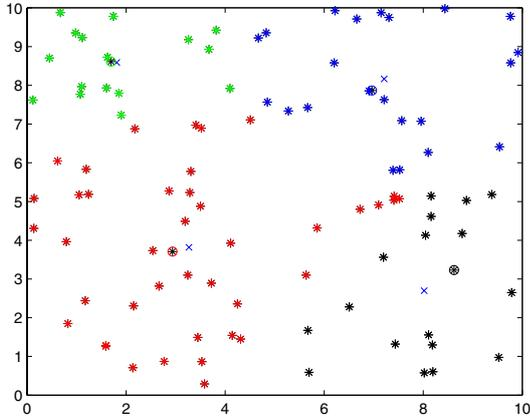
Fig. 2. A network topology generated by the described algorithm. Different colours of the client nodes, mark different piconets. Blue crosses mark the exact centres of gravity and the circled stars the PNCs.
