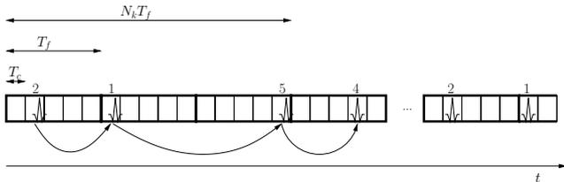
Fig. 1. Illustration of some parameters used in the system model. In the example  $c^{(k)} = (2, 1, 5, 4)$ ,  $d_1 = 1$  and  $d_2 = 0$ .
