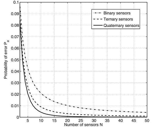
Fig. 6. Probability of error  $P_e$  of Chernoff information-based serial networks with binary, ternary, and quaternary sensors at observation SNR of 6 dB.
