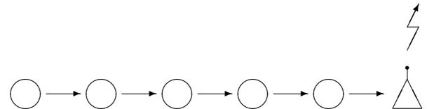
Fig. 1. Linear wireless sensor network with gateway node.
