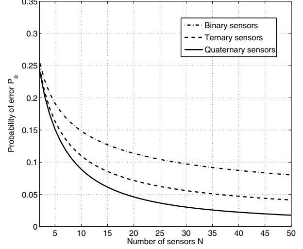
Fig. 4. Probability of error  $P_e$  of Chernoff information-based serial networks with binary, ternary, and quaternary sensors at observation SNR of 0 dB.
