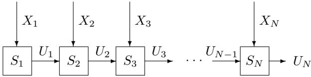
Fig. 2. Serial distributed detection system.
