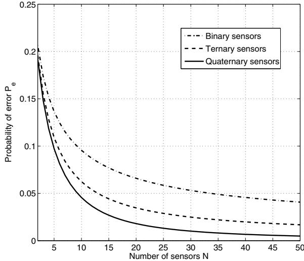
Fig. 5. Probability of error  $P_e$  of Chernoff information-based serial networks with binary, ternary, and quaternary sensors at observation SNR of 2 dB.
