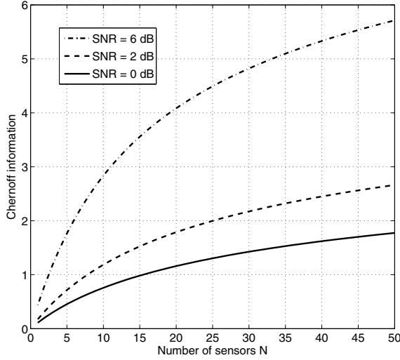
Fig. 3. Chernoff information in serial networks consisting of quaternary sensors as a function of the number of sensors for varying observation SNR.
