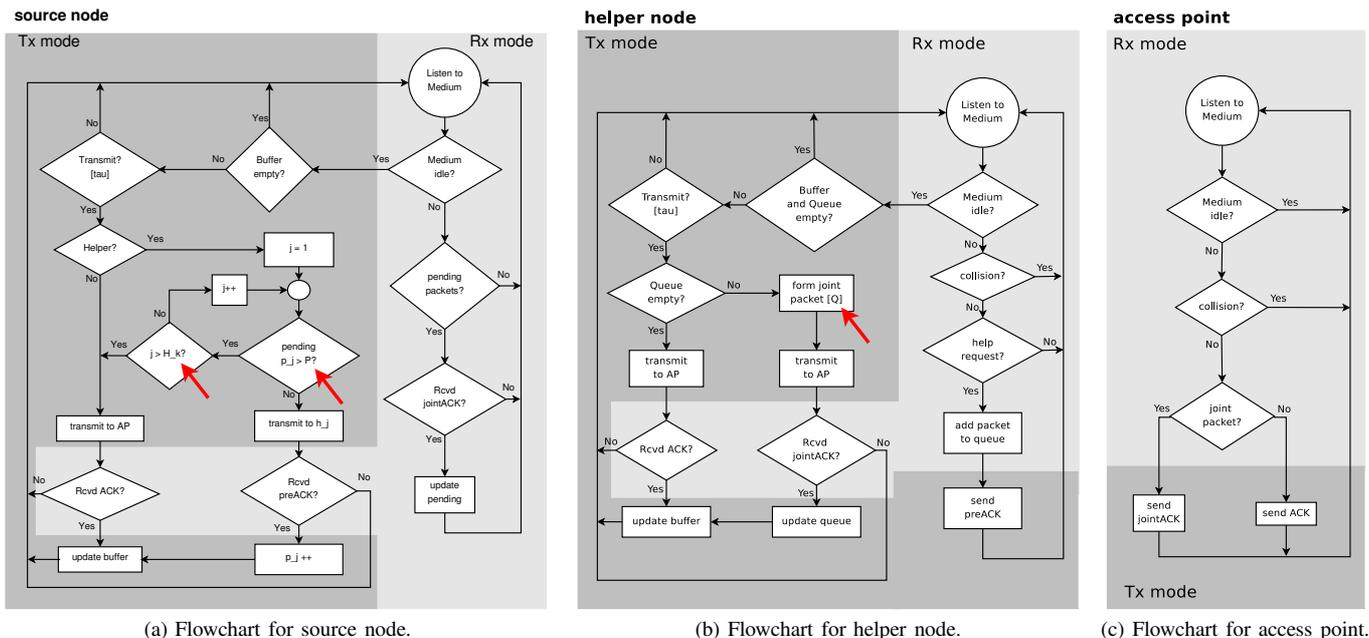
Fig. 2. Flowcharts for fairMAC as described in Subsection IV-B. The parameters maximum number  $H_k$  of helpers, maximum number  $P$  of pending packets per helper, and the maximum number  $Q$  of packets forwarded at a time are emphasized by an arrow.
