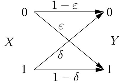
Fig. 5. The binary asymmetric channel with error probabilities  $\varepsilon, \delta \in [0, 1]$ .
