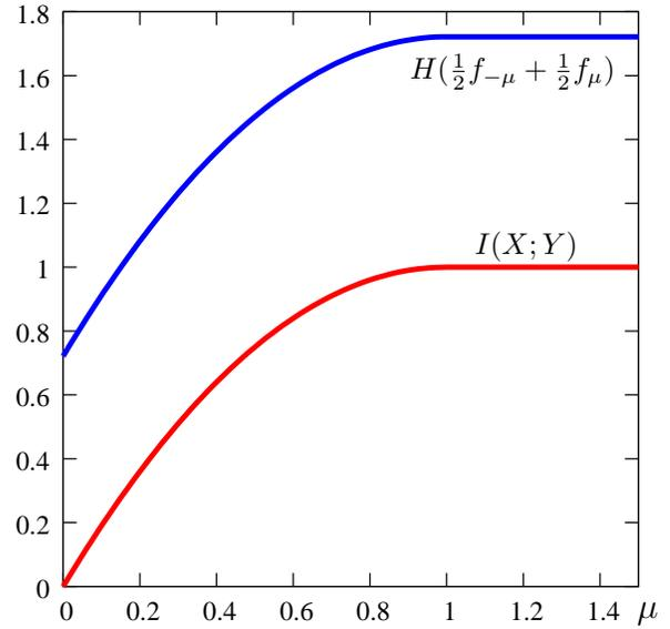
Fig. 2. Entropy and mutual information of a channel as a function of  $\mu > 0$  with the triangular as noise distribution and 2-PAM signaling points  $-\mu$  and  $\mu$ .
