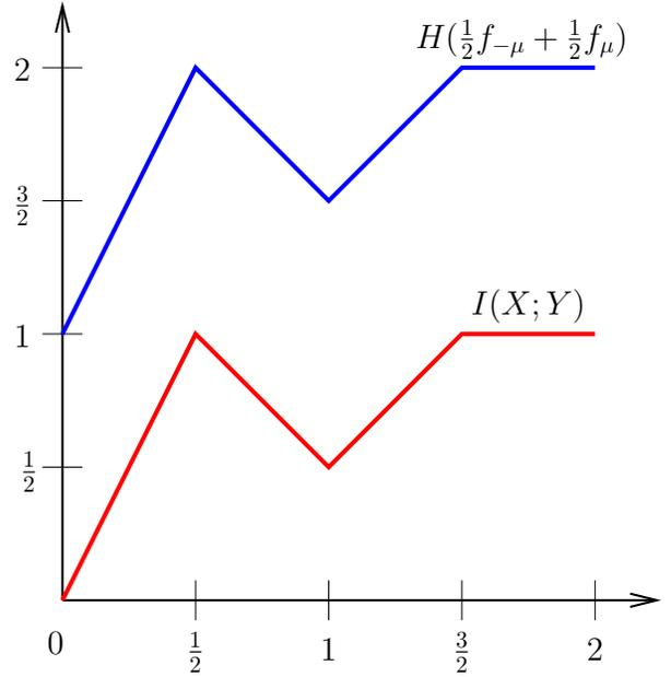
Fig. 4. Entropy and mutual information of a channel as a function of  $\mu \geq 0$  with segmented uniforms as noise distribution and 2-PAM signaling points  $-\mu$  and  $\mu$ .
