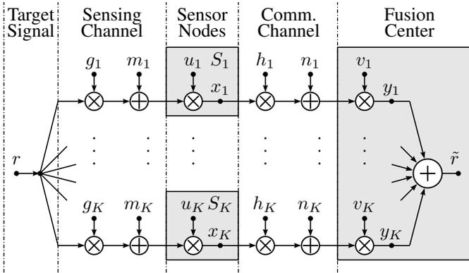
Fig. 2. System model of the distributed sensor network.
